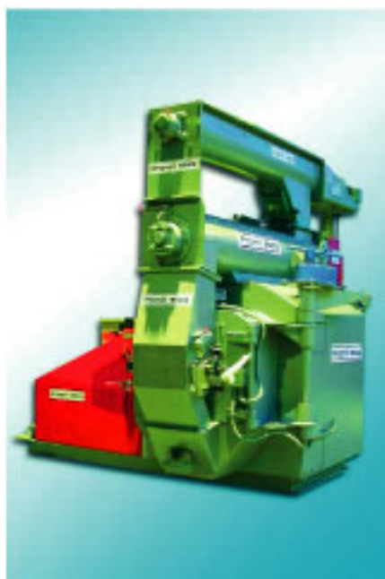
Pelletising mill for animal feed
